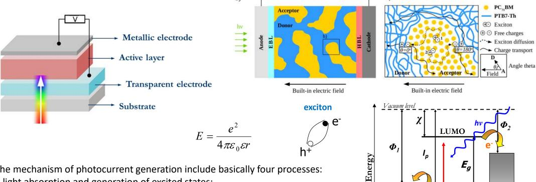
The mechanism of photocurrent generation include basically four processes:
