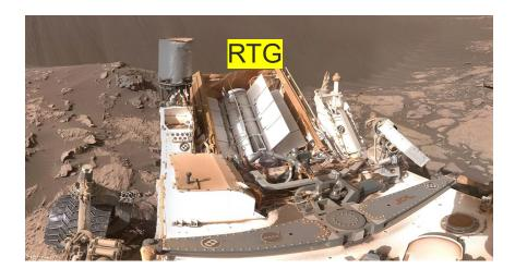
RTG is the only steady power supply for space probes running for over 30 years.
